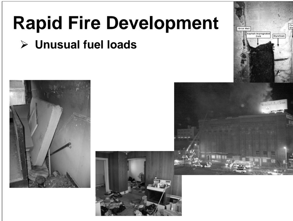
Fires in vacant or abandoned buildings may grow and develop in unusual ways due to heavy fuel loads in the building, exposed structural components, voids created by the removal of equipment and building systems, and the elements and vandalism.
