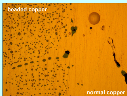
Figure 6. After polishing, there are impurities in the internal part of the bead. It is clearly different from the normal copper conductor. (500X)
