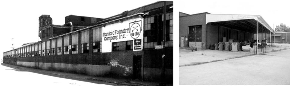
The use of a structure will provide the evaluator with clues to potential hazards that may be present. Industrial buildings like the one shown on this slide may have pits and shafts for machinery as well as potential hazardous materials including asbestos, PCB's in transformers, or oil contamination.
