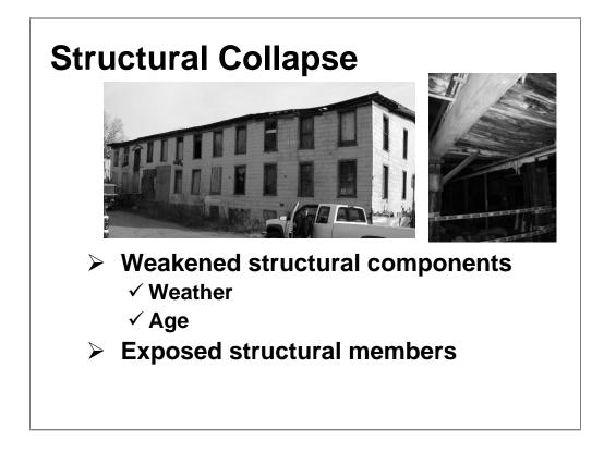
Structures that are weakened by vandalism, the removal of equipment or exposure to the elements are likely to collapse with out warning. Under fire conditions the buildings may fail very rapidly as already weakened structural elements are consumed.
