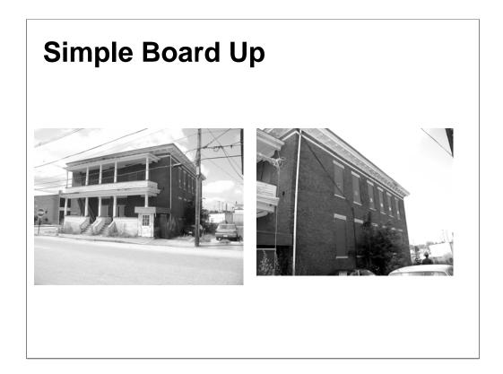
This slide shows an example of a non-reinforced board-up of a historic structure. Note vents and light panels on upper floors. This is the least complex and lowest cost method for securing a structure. It is also the easiest to breach.
